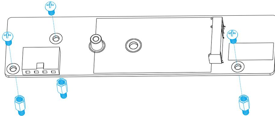
4. Insert the SSD at a 45 degree angle, make sure the notch meets (indicated by the **blue circle**). Gently lower the other end of the SSD and secure it with a screw.
