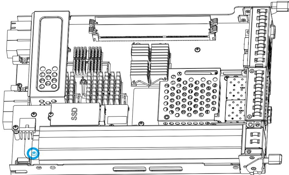
3. Lift the Super Capacitor from the screw end at 45 degree angle.
