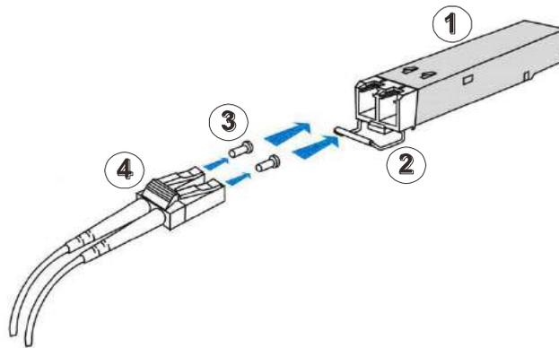
3. Insert the SFP module into the system host ports. The module will click into place.
