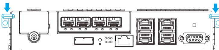
5. **Insert the new controller module.** Carefully push the controller until you feel the contact resistance when the board edge connectors are engaging the backplane. Push the ejection levers upward (indicated by the **blue arrows**) and fasten the retention screw on the ejection levers.
