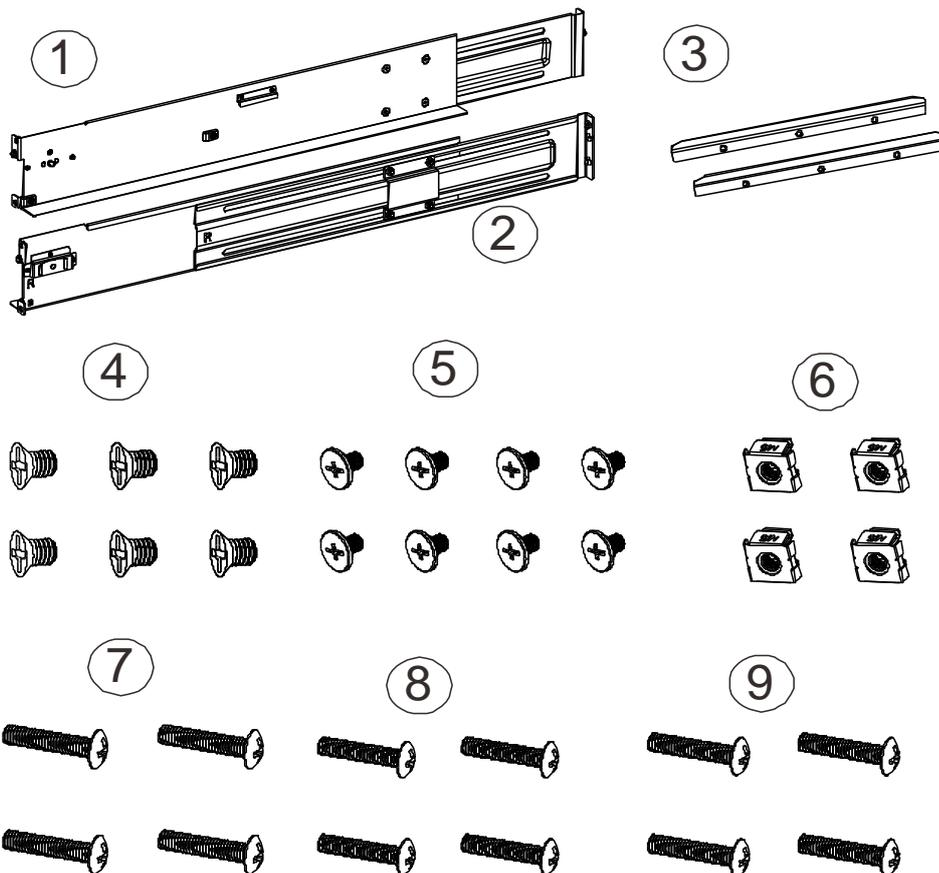
1. The installation begins with determining the installation position (front and rear rack positions) and M5 cage nut (5) insertion location.
