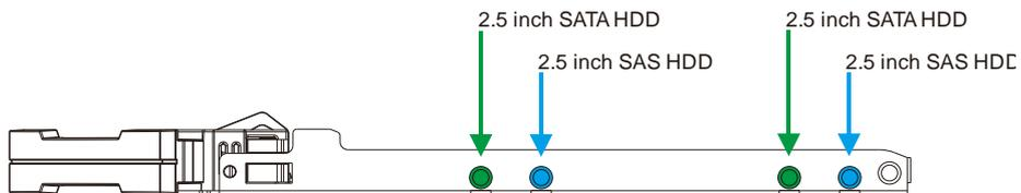
Adjust the drive location until the mounting holes in the drive tray are aligned with those on the hard drive. Secure the drive with four of the supplied flat-head screws.
