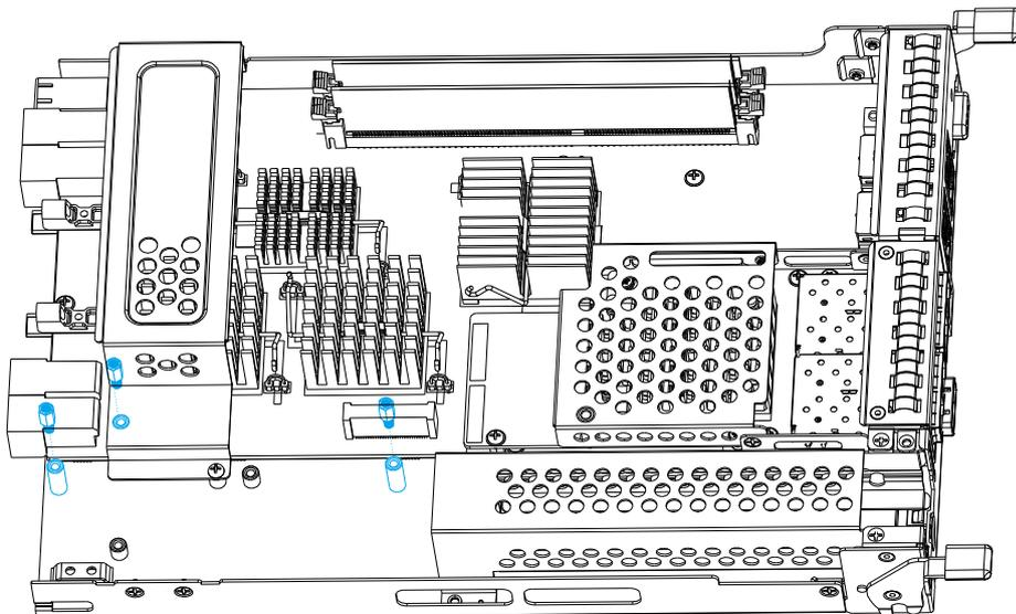
3. Make sure the screw holes meet while placing the SSD PCB board on the copper stands. Secure the PCB with screws provided.
