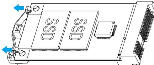
4. Insert the new FBM on a 45 degree angle, make sure the notch matches and gently push the end downwards till the clips clamp on.
