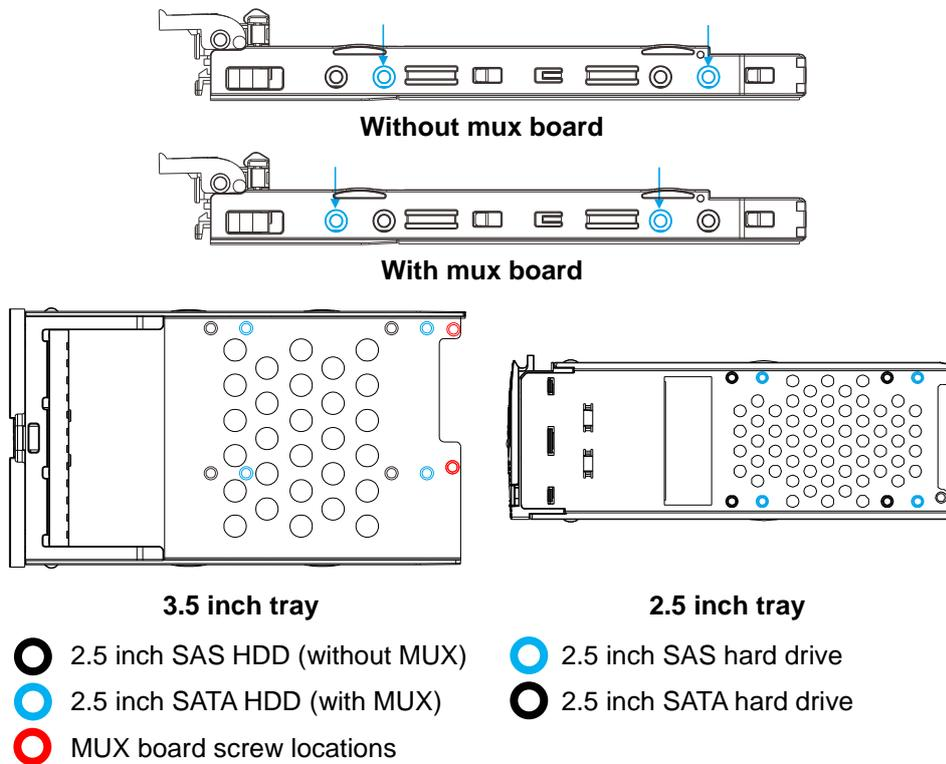
6. **Replace the drive.** After swapping the drive, fasten the retention screws back. Refer to screw locations in the previous step.
