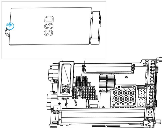
3. Insert the replacement flash backup module on a 45 degree angle, gently lower the other end of the SSD and secure it with the original screw.
