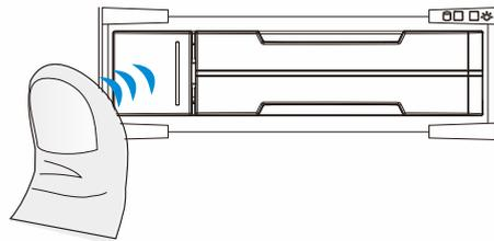
3. **Remove the drive tray.** Pull the tray one inch away from the enclosure. Wait for at least 30 seconds for the disk drive to spin down, and then gently withdraw the drive tray from the chassis.
