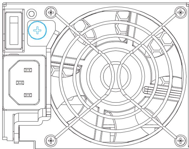
3. To remove the PSU module, pull the extraction handle downwards to disconnect the PSU from the backplane connectors. Once dislodged, gently pull the PSU out of the system. If the system is mounted in a rackmount rack, use another hand to support its weight while removing the module.
