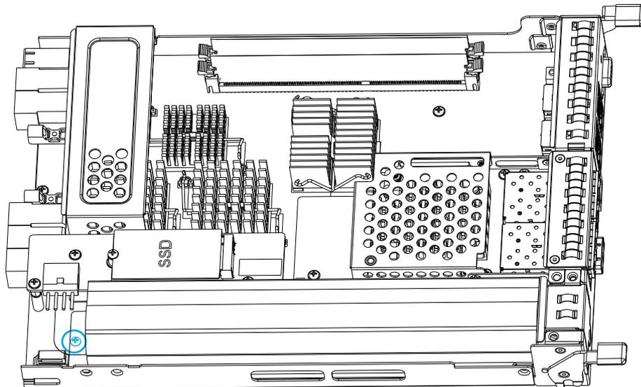
3. Connect the four-pin molex connector to the SSD PCB board.
