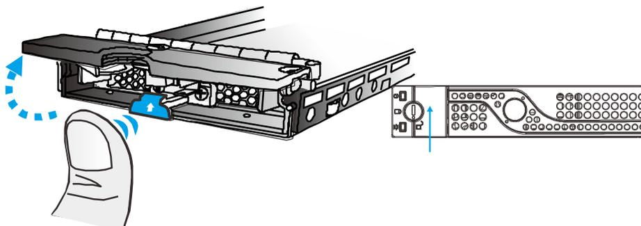
4. **Remove the drive tray.** Pull the tray one inch away from the enclosure. Wait for at least 30 seconds for the disk drive to spin down, and then gently withdraw the drive tray from the chassis.
