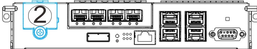
3. Install the replacement BBU module and fasten the thumb screw.
