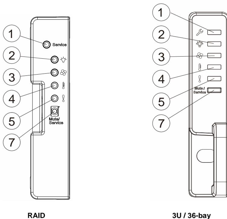
The LED panel on a JBOD storage expansion system can be located on the chassis ear. The LED panel contains Service LED (1), a power supply status LED (2), cooling module status LED (3), temperature sensor status LED (4), System fault LED (5), rotary ID switch (JBOD) (6) and a Mute Service button (7). For details, please refer to [LED Panel](#).
