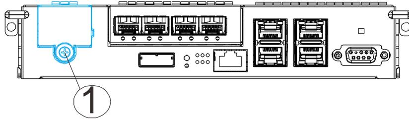
2. Using the thumb screw as an anchor, gently pull out the BBU **(2)**.
