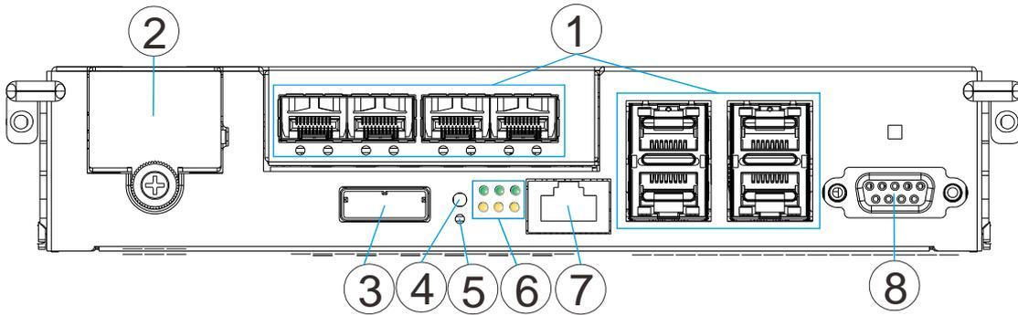
The controller on the dual controller models also features a **Cache Backup Module (CBM)**, consisting of a **Battery Backup Unit (BBU)** and **Flash Backup Module (FBM)**. The CBM and its components may be optional items for some systems.
