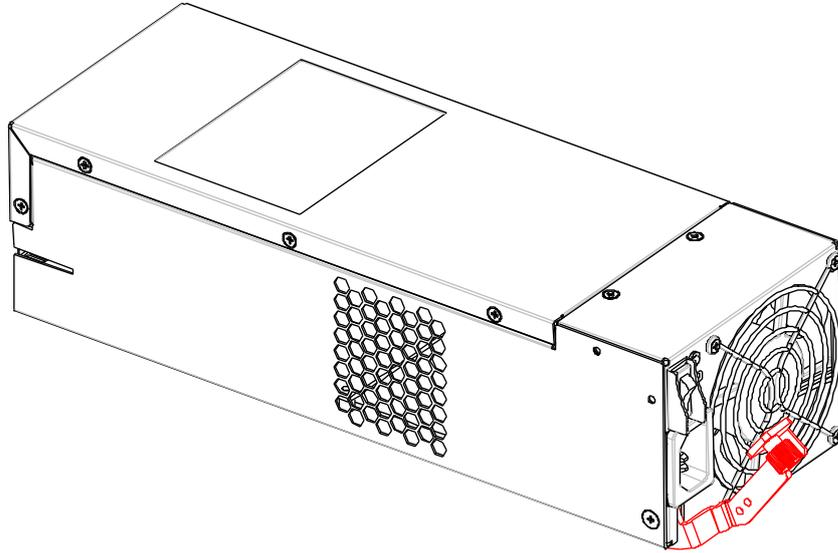
4. Insert the replacement module. Make sure the extraction handle is pointing outwards. Push the replacement PSU into the chassis, and when you feel the contact resistance, push the extraction handle towards the PSU module and it should engage the back-end connectors.
