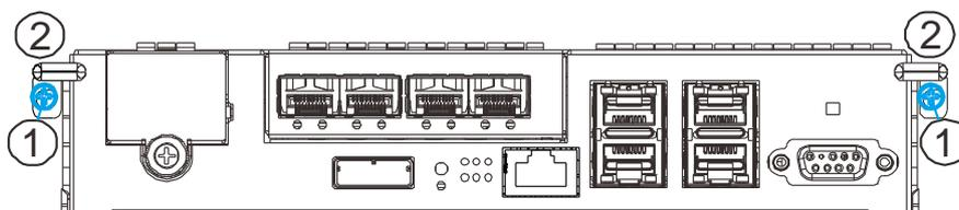
Push ejection levers downwards and the controller will ease out from chassis.
