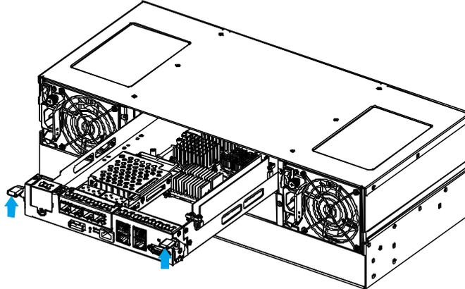
2. Secure the controller by fastening the two retention screws **(1)** under the ejector levers **(2)**.
