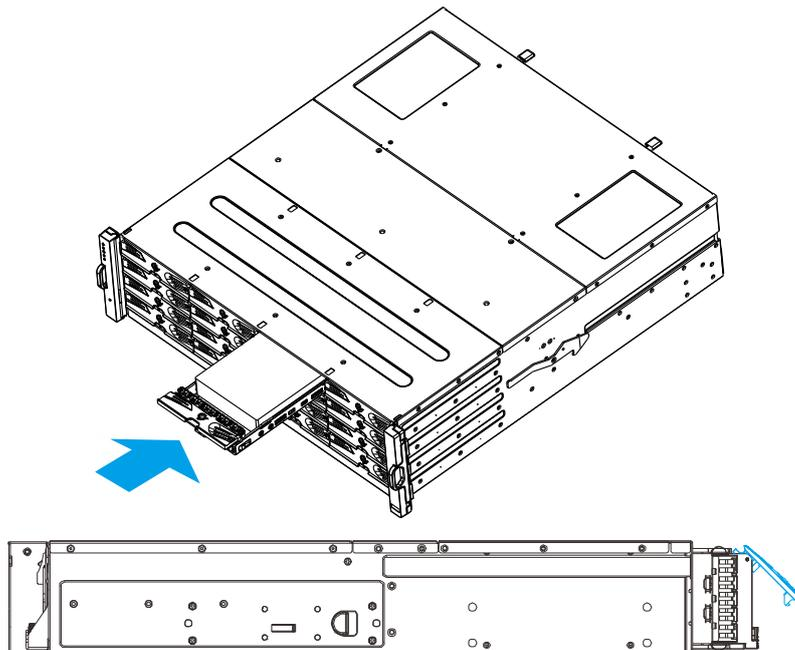
8. **Lock the drive tray.** Turn the bezel lock to the vertical orientation (locked position) using a flat blade screwdriver. Do not push the bezel lock while turning it, otherwise the spring handle will pop out again.
