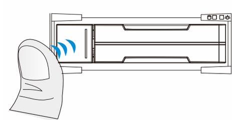
Place the hard drive into the drive tray, making sure that the interface connector is facing the open side of the drive tray and its label side facing up.
