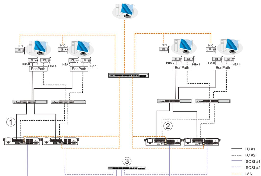
The above diagram demonstrates how to utilize the iSCSI host ports for remote data replication.
