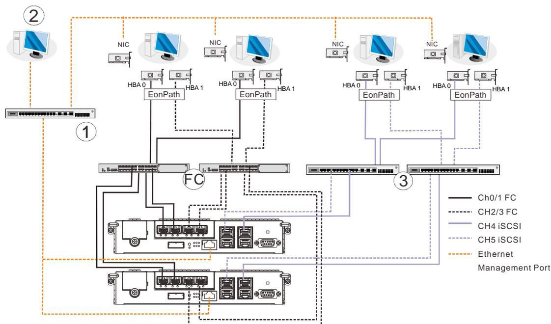
When connected to both FC host and iSCSI host, the connections will work in their respective speeds. It maximizes the number of connections while keeping the optimum performance gained by the high speed FC link and FC switch (**FC**).
